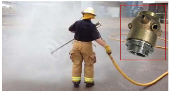
Piercing Rod System with Rotating Misting Head (close-up inset)
