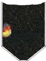
Thermal imaging camera identifies and locates the burning coal in the silo.
