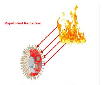
The encapsulating agents create a thermal circuit, where heat is drawn into the inner part of the droplet.
